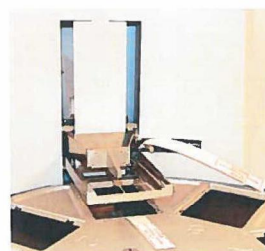
Figure 31 Both transport locks refitted
